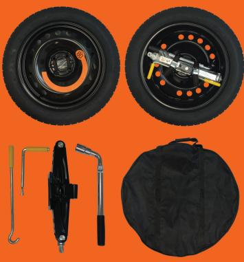
EACH ROADHERO SPACE SAVER WHEEL KIT IS ENGINEERED FOR A SPECIFIC VEHICLE FITMENT, NOT SOLELY RELYING ON PCD & OFFSET, BUT ALSO ALLOWING FOR BRAKE CALIPER CLEARANCE (X-FACTOR ETC). THE WHEEL & TYRE SIZE COMBINATION ARE ALSO SPECIFIC TO THE VEHICLE AND EACH KIT WILL EITHER BE DIRECT-FIT, OR BE SUPPLIED WITH THE NECESSARY FIXINGS TO ENSURE A PERFECT FIT.
